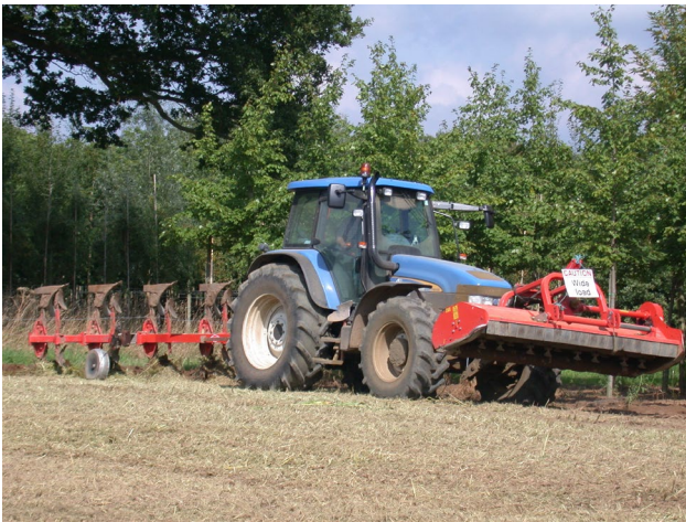
Figure 2 - Plough and mower used for incorporating Sudan grass
